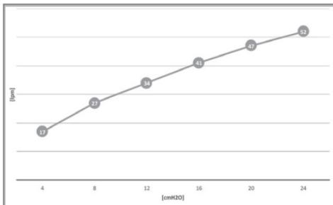
\*Due to machining differences, the outflow from the exhalation orifices may vary ( $\pm 10\%$ ).
